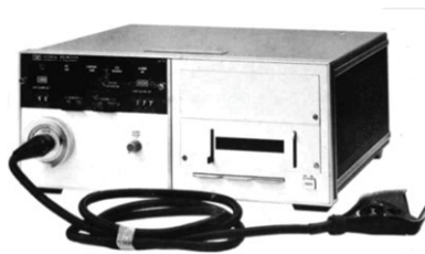
Figure 3: Hewlett Packard multi-wavelength ear oximeter
