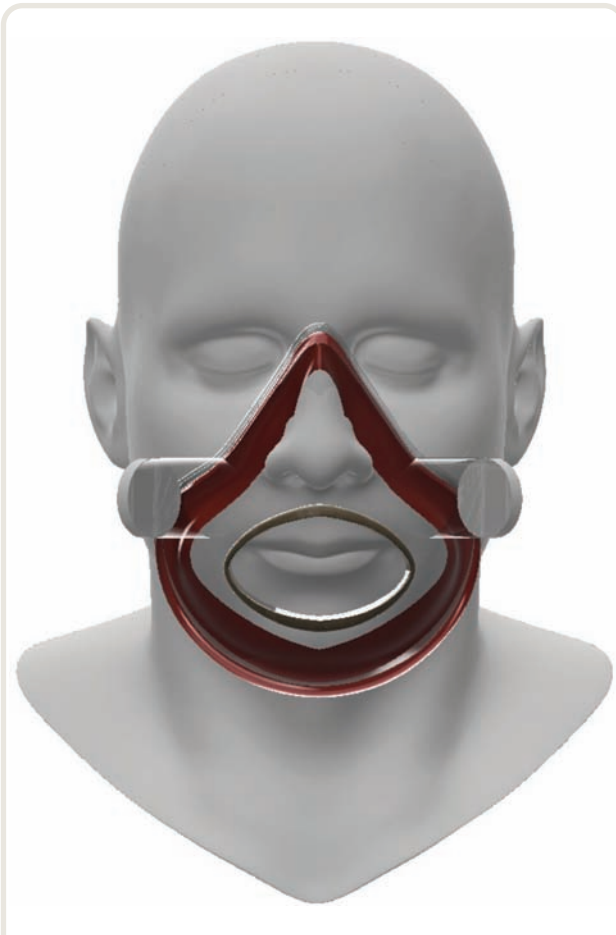
Fig. 4. Artist's conception of improved elastomeric respirator, with filter ports on either side of the respirator facepiece; the filters are deliberately not shown. The respirator body is transparent, and there is a speaking diaphragm to facilitate communication. The respirator would accommodate a wide variety of filters through the use of adapters, which could make the respirator more suitable to surge situations in which the supply chain for filters could be interrupted. The sealing surface is highlighted. There is no exhalation port; inhalation and exhalation take place through the same filters. Straps that hold the respirator onto the face are deliberately not shown, but are an important feature for fit and comfort. In the United States, respirators are certified for use by the National Institute for Occupational Safety and Health (Washington, D.C.); thus, the National Institute for Occupational Safety and Health would need to be involved in improved elastomeric respirator design.
