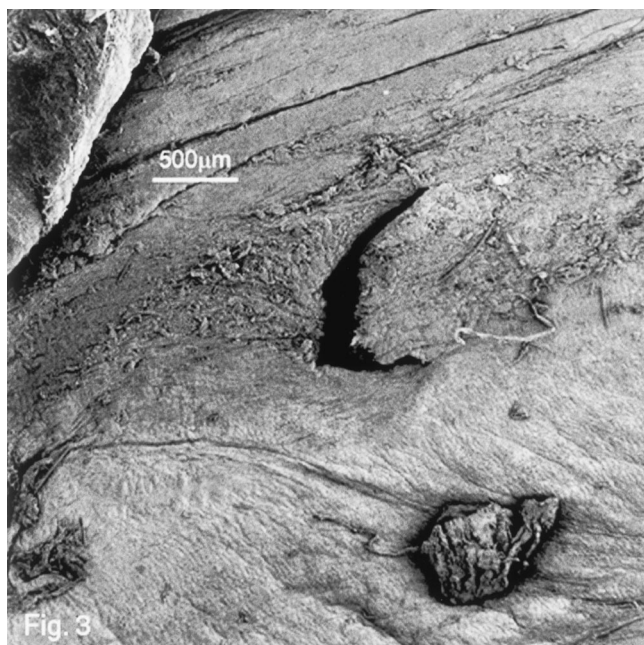
Fig. 3. Scanning electron microscopic image of a dural puncture made by an 18-gauge Tuohy-Schliff Perifix epidural needle with the bevel perpendicular to the dural long axis (90° angle).
