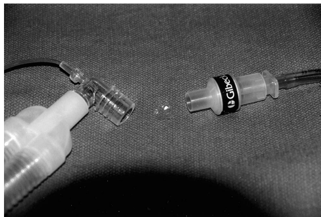
Fig. 1. A piece of plastic from a warm air blanket found lodged in a heat moisture exchanger.
