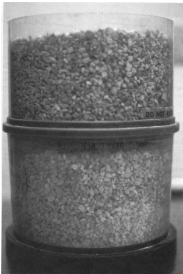
Fig. 2. Although this black and white photograph fails to demonstrate the dramatic color difference between the upper and lower compartments, carbon dioxide absorbent in the upper compartment is blue, suggesting exhaustion of the carbon dioxide-absorbent granules. No color change is seen in the bottom compartment because of the yellow tinting of the transparent plastic absorbent canister. The yellow plastic gives the granules a white appearance.
