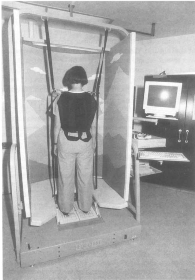
Fig. 1. The computerized dynamic posturography system (EquiTest; NeuroCom International, Clackamas, OR). The subject is seen standing on the hinged footplate facing into the three-sided visual surround ready for testing.
