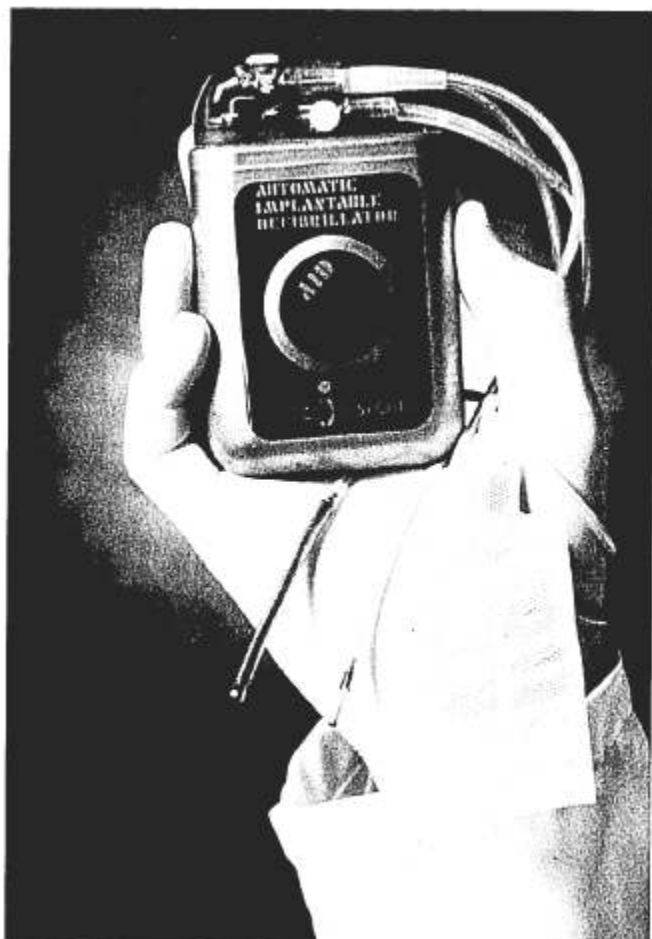
FIG. 1. The AID-B ® device with associated electrodes. The spring electrode on the left is one of the two defibrillating electrodes and is placed in the superior vena cava. The other defibrillating electrode is the patch on the right of the photograph, which is sutured to the cardiac apex. In the center is one of the endocardial electrodes placed in the right ventricle for rate sensing (photograph courtesy of Intec Systems, Inc., Pittsburgh, Pennsylvania).
