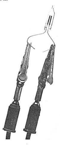
FIG. 1. Neon lamp (type NE-2) attached to clips from peripheral nerve stimulator.
