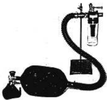
FIG. 1. Assembly of "PUFFA" showing modified reservoir bag connected by corrugated breathing tube to breath-through type vaporizer regulated and calibrated for halothane.
