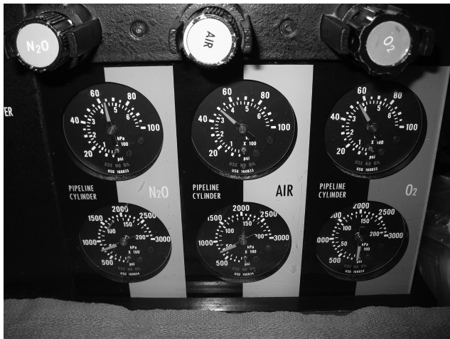
Fig. 3. The Narkomed 2B anesthesia machine medical gas pipeline gauges (Dräger Medical, Inc. Telford, PA) with the nitrous oxide line connected to the carbon dioxide wall gas outlet. Note that the nitrous oxide gauge is reading 62 psig, which is higher than one would expect if the line were connected correctly to the nitrous oxide wall outlet.
