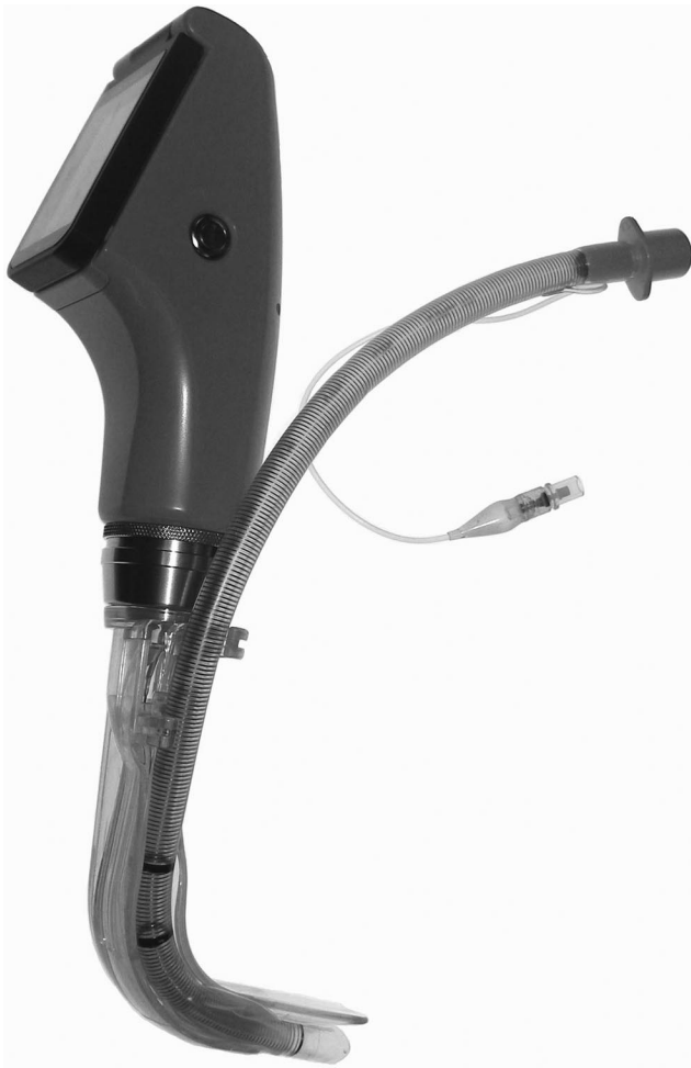
Fig. 1. The Pentax-AWS® (Hoya Corporation, Tokyo, Japan). It consists of a disposable transparent blade (PBlade®; Hoya Corporation), a 12-cm image tube with a charge-coupled device (CCD) camera, and a handle with a 6-cm full-color liquid crystal device monitor display.
