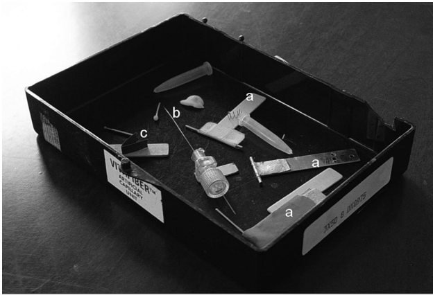
Fig. 1. I kept the old box that held the amicon microdialysis tubes. All along I used the box for all the small accessories that I needed for the experiments. I have only a few (and worn!) gadgets left; a = custom made devices for securing (via the stereotaxic device) the microdialysis fiber and internal stylet; b = spinal needle stylet attached to one of the devices; c = small piece of sandpaper that I used to clean off the stylet after use (epoxy occasionally got stuck during the processing).
