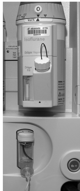
Fig. 1. Dräger Apollo anesthesia machine with water trap located directly below the isoflurane vaporizer.
