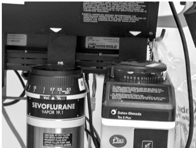
Fig. 1. Photograph showing detail of vaporizer-selection system malfunction. The vaporizer activation indicators are both illuminated. The photograph was taken after the event, and the set vaporizer readings do not reflect the concentrations used in the incident.
